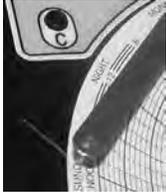
Chart recorder stylus and time line groove
