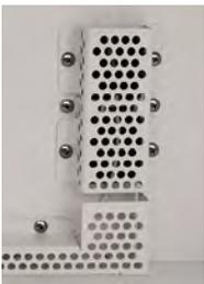
*Chamber temperature sensor (located behind cover).*
